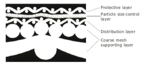
Cross section Structure of sintered mesh filter (different products have different layers)
